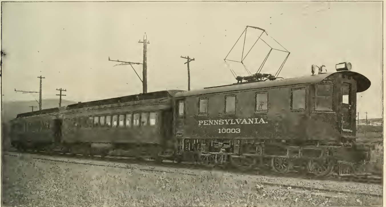
ELECTRIC LOCOMOTIVE WITH FRAME LIKE THAT OF A STEAM LOCOMOTIVE. HIGH CENTRE OF GRAVITY.
